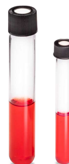
b. Comparison between Solstice (8 mL) and Solstice MAXI (20 mL) tube reactors
