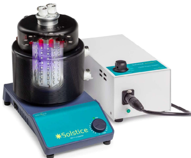
Solstice with 120W Borealis LED module inserted
