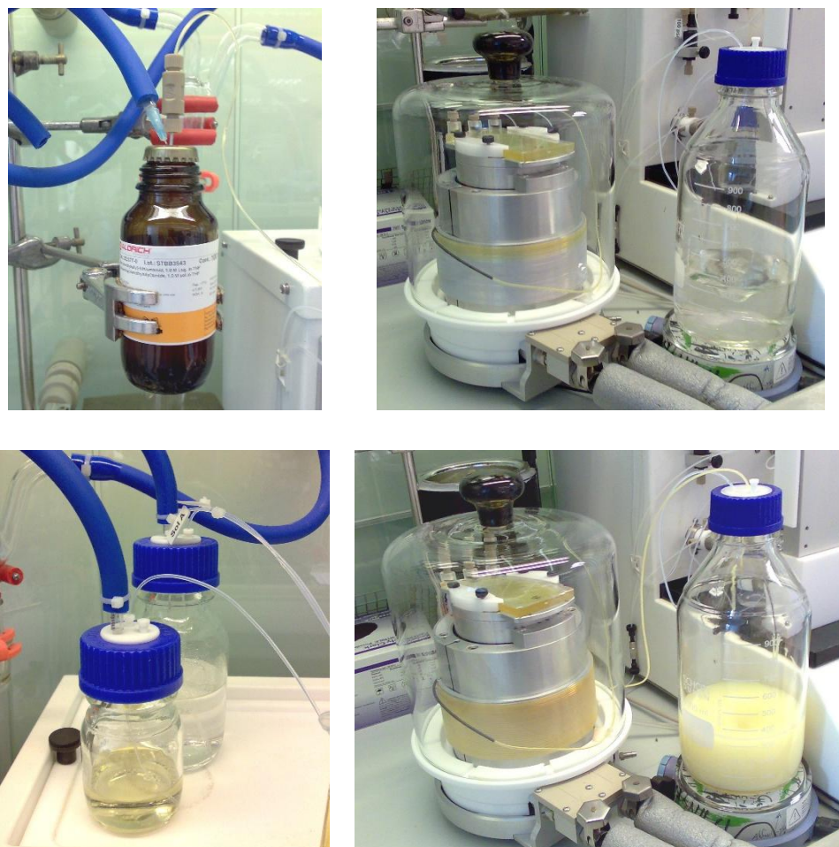
Figure. Preparation of intermediate 3 using FlowSyn fitted with a 'Cold Coil' and Static Mixer Chip.
