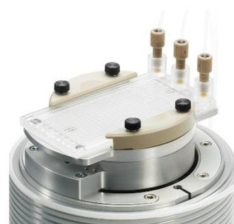
Since the Cold Coil is a true standalone module with no internal electronic control components it can be readily assimilated into an existing flow reactor system. Alternatively, several units may be quickly connected in series to afford a rapid route to scale-up.
