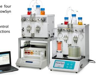
As a stand-alone reagent delivery module, the **BPM** is controlled using user-friendly PC software and can act as a core component for a modular flow reactor system. For performing single experiments up to 4 reactor modules can be added choosing any combina on of **HotCoil**, **Cold** Coil and **Polar Bear Plus Flow** units.
