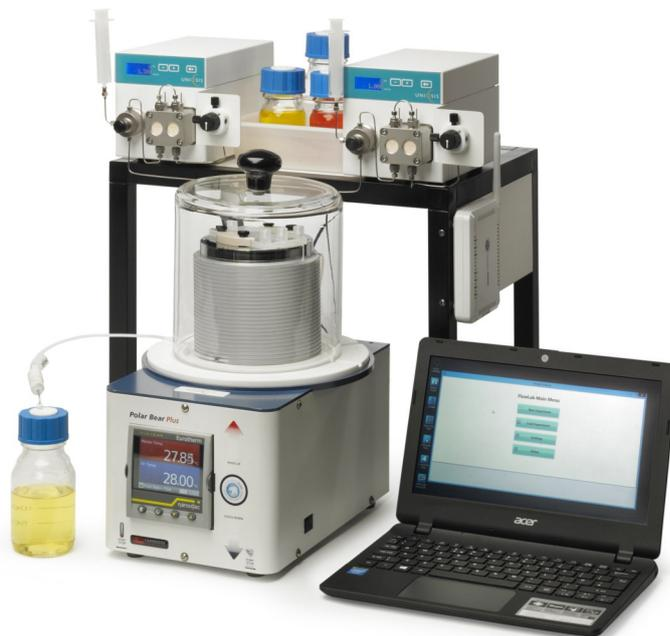
FlowLab Cold™ is based around the same core components as FlowLab but the HotCoil reactor module is replaced by the Polar Bear *Plus* Flow cryogenic module. This allows experiments to be performed from -40°C to +150°C. No liquid nitrogen or card-ice is required when operating in sub-ambient mode.
