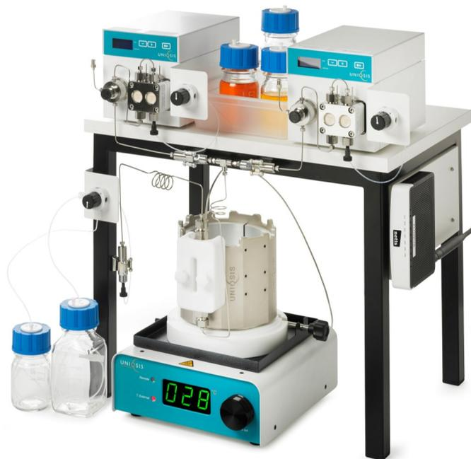
**FlowLab Column™** is an alternative configuration of the **FlowLab** system designed specifically for high temperature and pressure catalytic flow chemistry applications. At the heart of the system is a **HotCoil** heated reactor module fitted with a **HotColumn** adaptor. This can hold up to 6 stainless steel HPLC columns in individual insulated holders. This configuration facilitates scale up whereby the required number of identical columns are simply connected in series.
