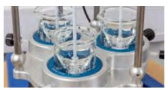
The Vortex Blend offers the scientist a compact space saving way of performing 3 blending experiments in parallel.
