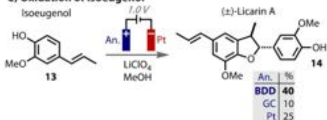
Figure 17. A) Two possible mechanisms for the oxidative methoxylation of 9 (a) and (b) to give 10 . Aldehyde 11 is formed from (c); B) ESR spectra reveal methoxyl radicals, leading to mechanism (b); C) formation of methoxyl radicals are more efficient on BDD anode in oxidation of isoeugenol.
