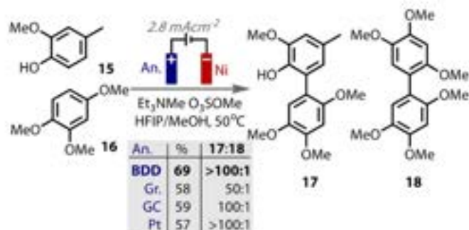
Figure 18. BDD gives best yields for phenol/arene coupling reaction, which produces reactive radical intermediates.
