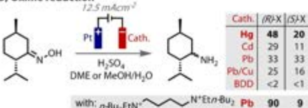
Figure 9. A,B) Cathode material with a high overpotential for proton reduction is necessary for attaining good selectivity for substrate reduction.
