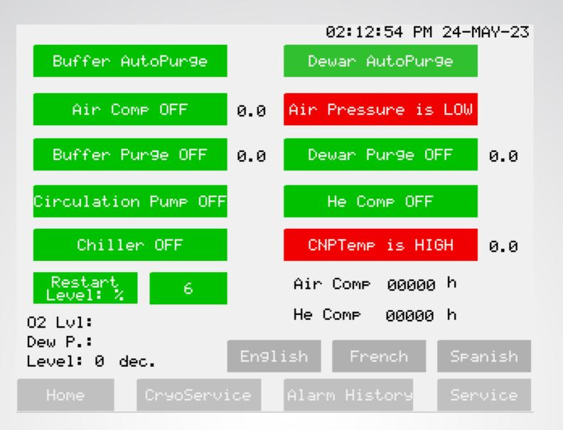
Experience enhanced accessibility and convenience with the CNP40's advanced PLC screen interface. This innovative system not only centralizes control and offers comprehensive monitoring capabilities, but it also enables remote monitoring from your personal computer! Moreover, the Diagnostic's Screen pictured above allows for monitoring of the Air Pressure in the Air Compressor and Buffer Tank as well to ensure safe operation.
