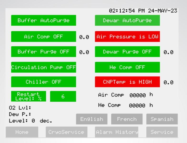
Experience enhanced accessibility and convenience with the CNP30's advanced PLC screen interface. This innovative system not only centralizes control and offers comprehensive monitoring capabilities, but it also enables remote monitoring from your personal computer! Moreover, the Diagnostic's Screen pictured above allows for monitoring of the Air Pressure in the Air Compressor and Buffer Tank as well to ensure safe operation.
