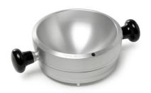
DrySyn MAXI features stand-alone bases for both 2000 mL and 3000 mL round-bottom Additional 2000 ml flask insert flasks. available for use with the larger base.
