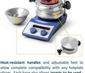
allow complete compatibility with any hotplate stirrer. Each base also allows **inserts to be used-one at a time** - to adapt it to accommodate additional standard flask sizes.
