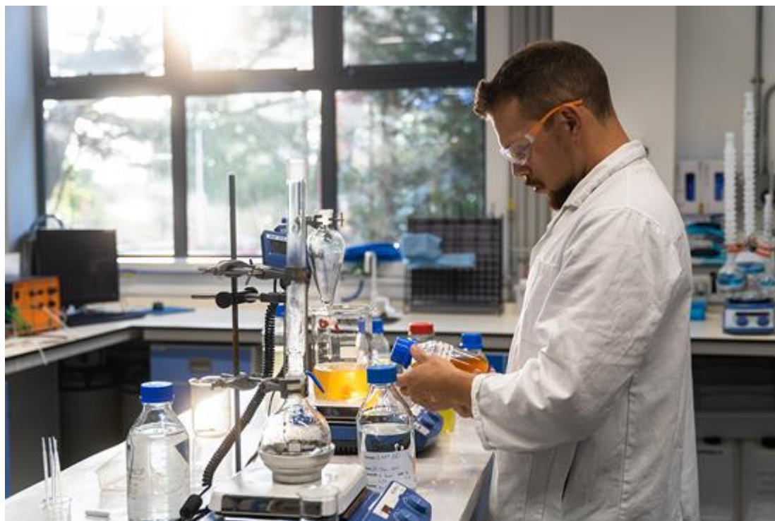
Caption: Dr Ed Jones carrying out small-scale reactions in DrySyn heating blocks
