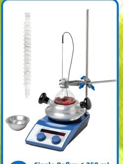
Single Reflux ≤ 250 mL 1 x DrySyn Scholar 250 mL Base, 1 x 100 mL insert to suit round bottom flasks, 1 x 350mm CondenSyn
