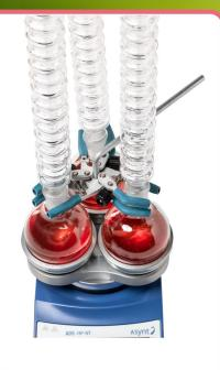
Parallel Reflux ≤ 250 mL 1 x DrySyn MULTI-M Base, 3 x each of 100 mL & 250 mL inserts to suit round bottom flasks, 1 x DrySyn MULTI-M 3 position clamp, 3 x 350mm CondenSyn
