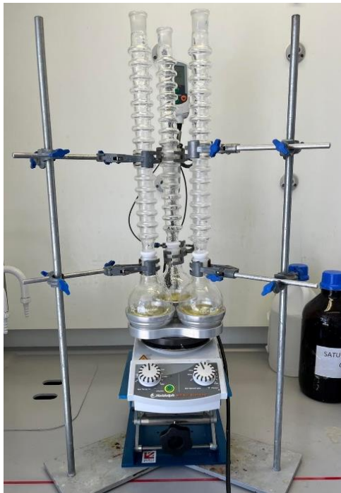
Caption: Students using DrySyn heating blocks and CondensSyn waterless condensers.
