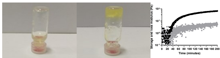
Figure 1 2 units of alkaline phosphatase (ALP) was added into 1 ml of 2% w/v (Napffk(AZT)Y(p)G-OH) solution (a), then it rapidly formed a gel (b) as confirmed by rheology. In the rheology time sweep (c), the value of storage modulus exceeds that of loss modulus at around 35 minutes, which indicated the gelation network formed at this time.
