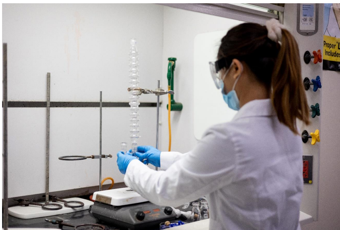
Caption: Margarete Teo, a student in the teaching labs at the College of the Sequoias (Visalia, CA) using the CondensSyn waterless condenser
