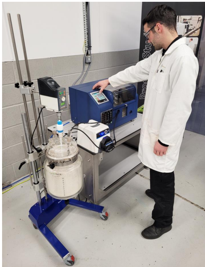
Caption: AMT clean room operation using a Coflore® flow reactor fed by an efficiently stirred vessel in a ReactoMate ATOM stand.
