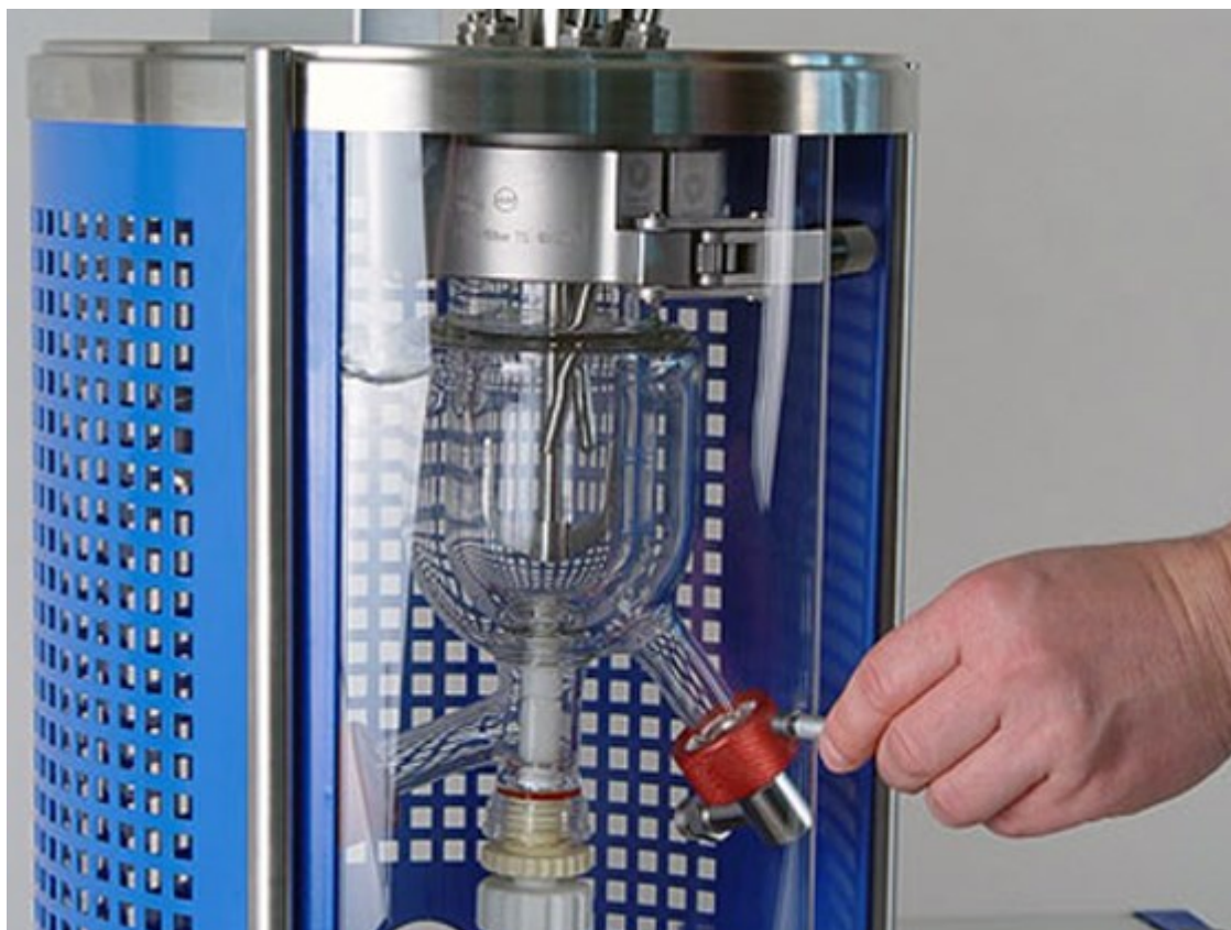
Compact lab reactor system for low and high pressure reactions, with interchangeable glass and steel pressure vessels (Picture: Büchi AG)
