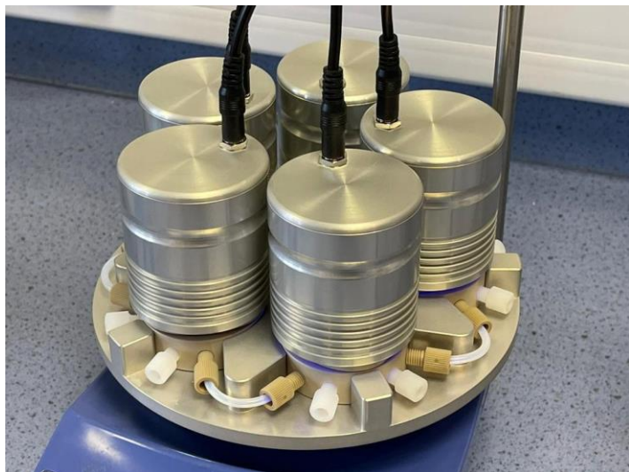
Caption: An Asynt fReactor Photo Flow with 5 modules set-up on a hotplate stirrer
