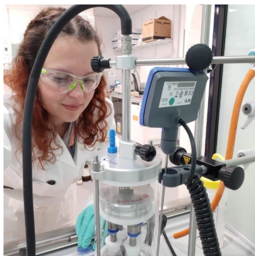
Caption: Virginie Viseur from the Kay Group operating the DrySyn Spiral Evaporator
