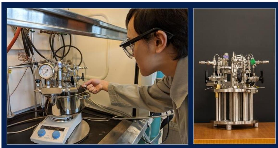
Caption: Custom Multicell high pressure parallel reactor in use.
