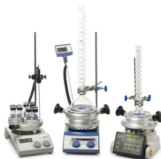
*All DrySyn® bases are supplied with adjustable feet to offer compatibility with any hotplate stirrer.*
