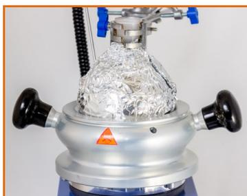
Insulating the flask reduces the thermal gradient across the glass thereby reducing stress on the flask at high temperatures.
