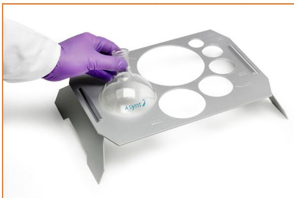
Use a gauge to check that your flask does not exceed the maximum size as specified by DIN ISO 4797.
