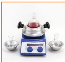
*With the DrySyn® heating blocks, the handles simply screw into the base.*
