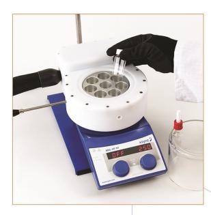
An innovative fluid-free cooling plate that enables rapid cooling of samples in vials or round bottom flasks (up to 500 mL) to below -60 °C.
