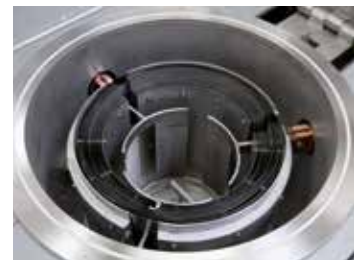
Cylindrical retort with tungsten heating
