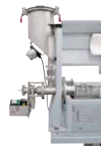
Vibration generator at the charging funnel for improved powder supply
