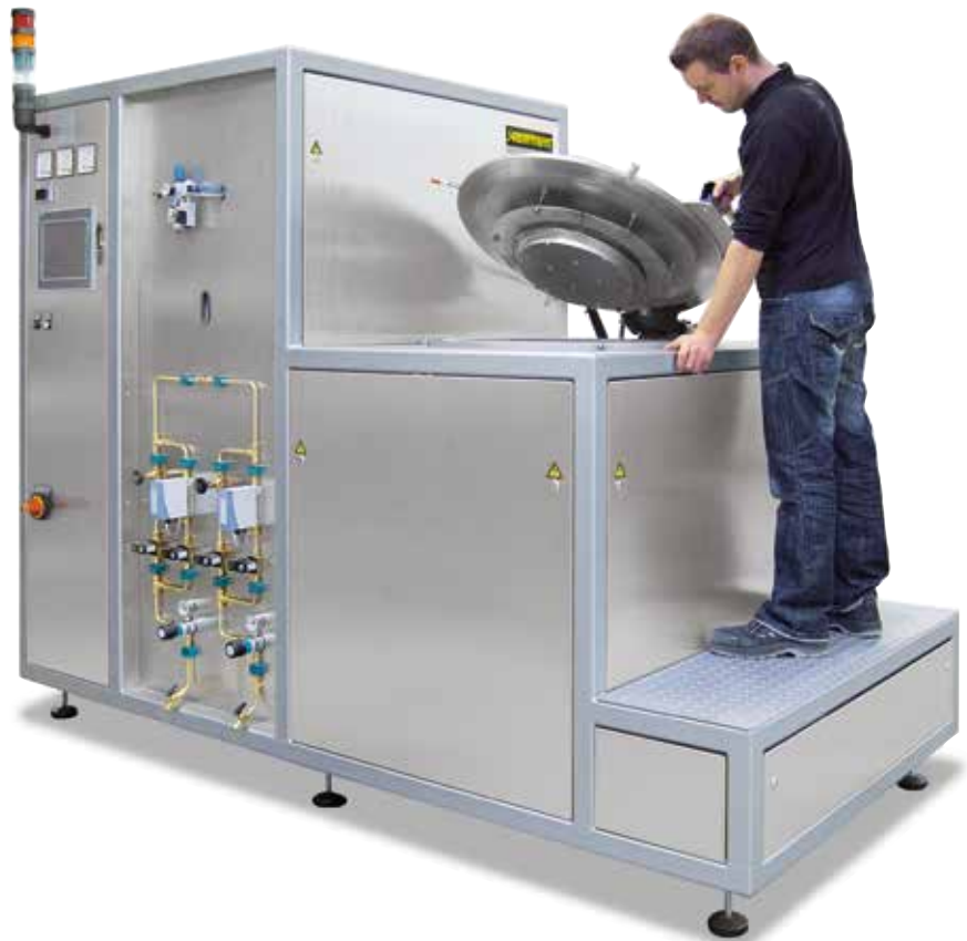
Retort furnace SVHT 9/24-W with tungsten heating
