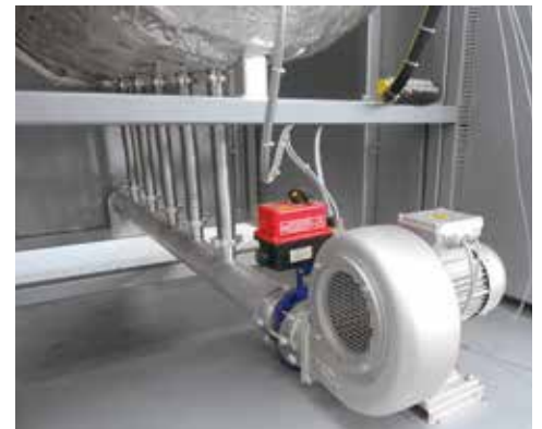
Fan cooling, hot-wall retort furnace NRA 400/03
