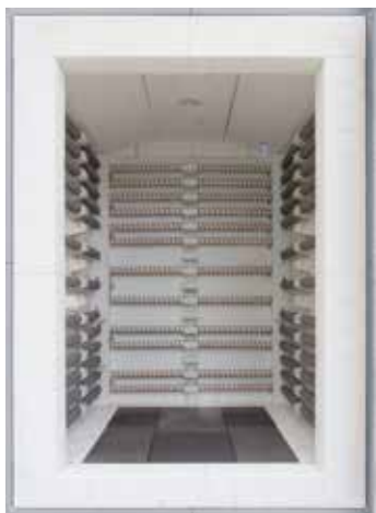
Chamber furnace N 650/14 BO with ignition burner
