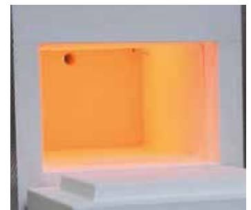
Muffle heated from four sides
