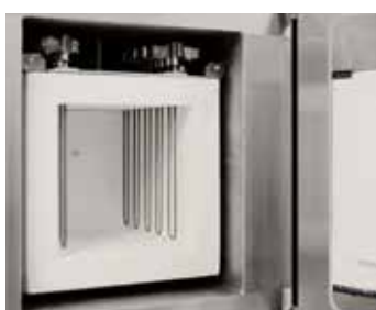
Molybdenumdisilicide heater and fiber insulation
