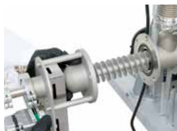
Screw-conveyor with adjustable speed
