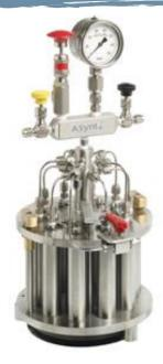
A cost effective, lightweight unit suitable for numerous stirred or non stirred applications. These include hydrogenations and applications where air sensitive materials are used or any other reaction where pressure or temperature are required.
