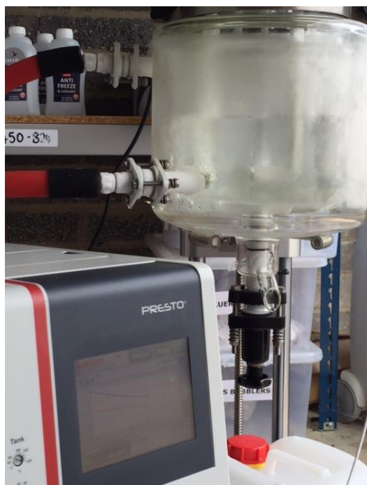
Picture 3: 5 litre vacuum jacketed reactor and Presto
