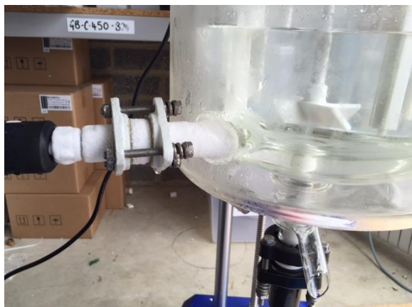
Picture 4: 5 litre vacuum jacketed reactor
