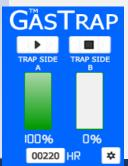
HYDROGEN LEAK DETECTOR - If outlet flow exceeds 300ml/min by >50% for more than 5 mins either hydrogen demand at GC/MS has been increased or a leak has occurred. An audible warning will sound and , if not reset in 10 mins (i.e. a temporary high flow demand) the hydrogen supply will be shut off.
