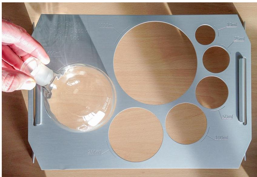
Ideally use a gauge such as Asynt DrySyn® Flask Size Gauge to check your flask conforms to the required ISO standard size
