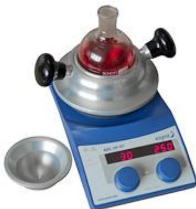
With the DrySyn® Heating Blocks, the handles simply screw into either side of the base
